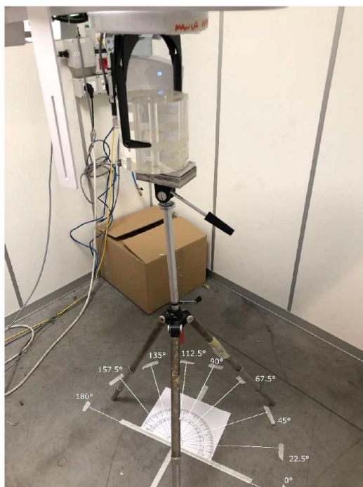
Experimental setting for stray radiation measurements in CEPH mode.
