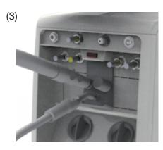
(3) Insert (2) into the connector. A vacuum connector cap (hereinafter, 'connector cap') should be attached to a connector that is not being used.
