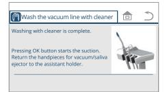
3. When you have finished washing the vacuum line with cleaner, press the  $\bigcirc o\kappa \bigcirc$  switch.
