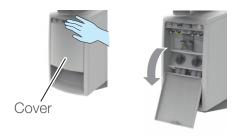
Maintenance panel cover Press the maintenance panel cover to open it.
