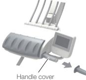
[Method to detach] Rod type Remove the handle cover. \* Be sure to remove it by hands.
