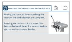
3. When you have finished rinsing the vacuum line+washing the vacuum line with cleaner, press the ок switch.
